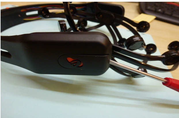
Fig. 7: Remove cover panels and unscrew sender-unit and accumulator
