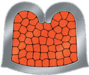
Fig. 19A: Crimping Profile
