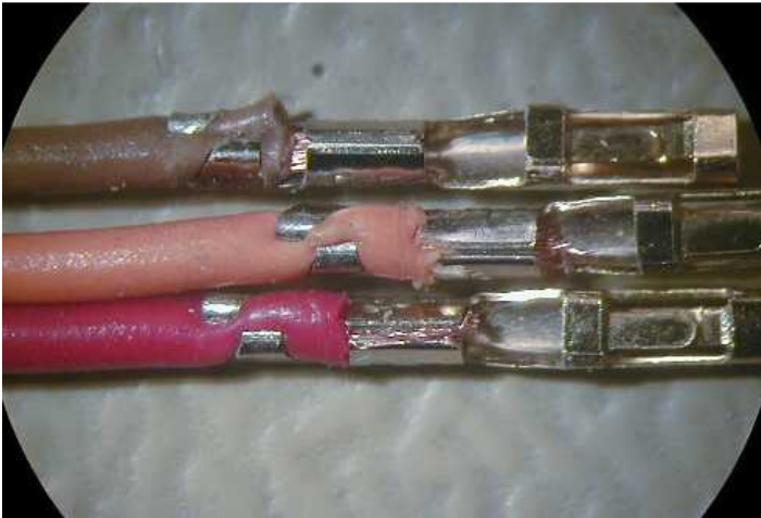
Fig. 19B: Crimped tension relief
